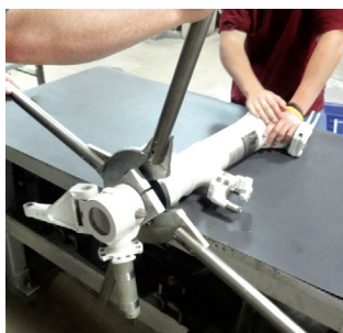
Hawker 400A Gland Nut Removal Tool
